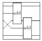
template for building a 2n-bit adder from two n bit adders.
